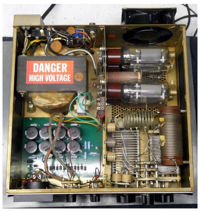
Remove tubes and loosen the fan to move it out of the way. The new choke installs first.
