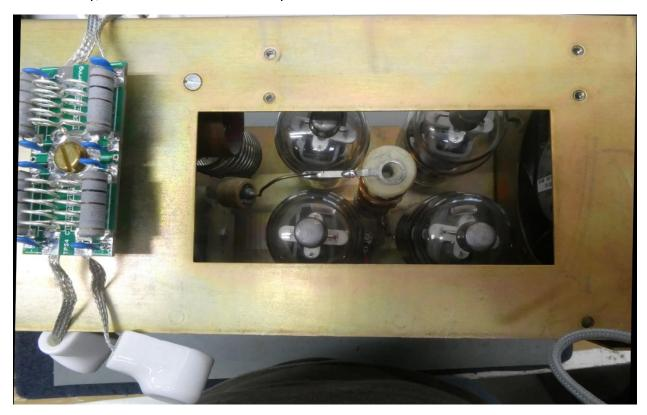
These are alternate connection points for the flying choke lead. If one of these holes is used for the enamel wire connection, be careful. Do not bridge to adjoining traces! The large center foil ring is the same connection spot as the two small pads:
