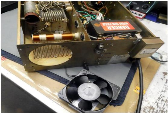
Having the fan out of the way allows much better access to the choke bottom connections. The choke connects the same way on the bottom:
