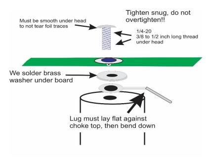
The long-lug in the RFC245LL choke kit can be used as shown for the choke wire connection. Alternatively, the choke wire can carefully attach to a hole in the TPS4:
