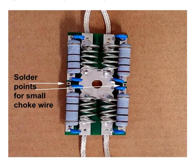
The installed choke and suppressor look like this (this Clipperton has filament GDTs and a hum balancing transformer). Be sure the braids to the white caps do not accidentally contact anything:
