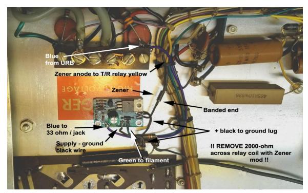
Note: The 2000-ohm resistor can be left in, but it is a pretty low value. While current is only around 60mA, this resistor dissipates 8-watts!
