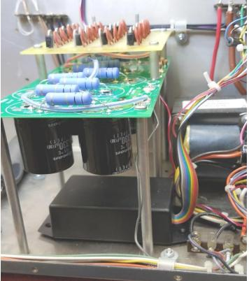
9.) The black rectifier negative Rect- and gray B- solder in last. The black rectifier wire can be trimmed to length or dressed around out of the way. Heavy Teflon sleeve protects the black wire and the red wires. The lead dress is not especially critical.
