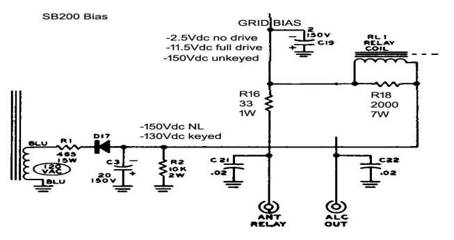
Control grids have the dominant effect on anode current. We never want ripple or anomalies in bias systems. Bias voltages should never waddle around with grid current with response rates slower than envelope modulation. This can cause IMD. (There are cases where bias can track RF envelope changes if in-phase and near audio or radio frequency rates, such as adding intentional negative feedback.)
