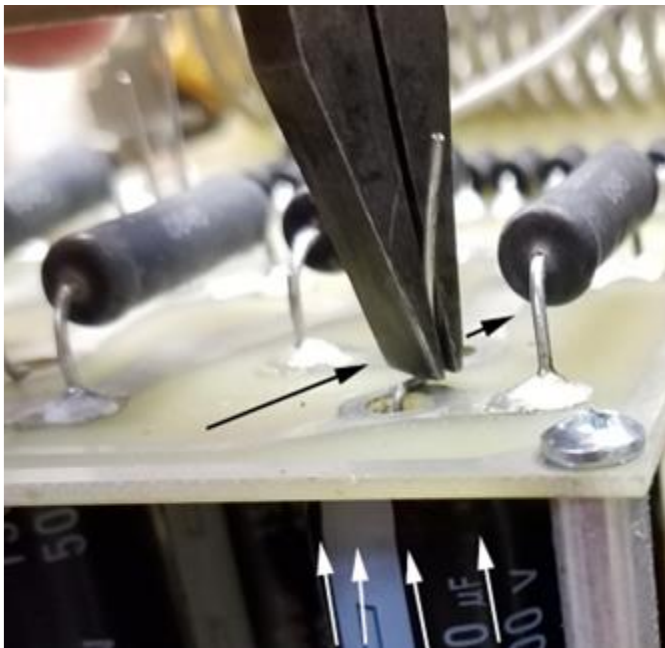
Figure 39 form leads to hold capacitors snugly
